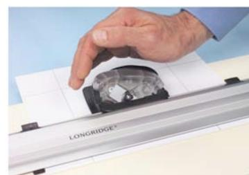
Manually retract the blade fully and take the cutter off the Guide Rail. The cutter stops of course remain set for the opposite long side (if cutting a rectangle and for the other three sides if cutting a square mount). Turn the mount around, check the pencil line against the Guide Rail and repeat the cut. Reset the bottom stop and repeat for the shorter sides if cutting a rectangular mount.
