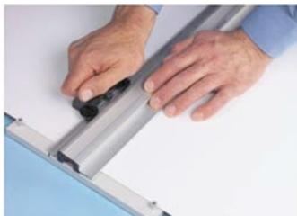
*be positive – don't hesitate, otherwise the blade may flex resulting in a curve at the end*
