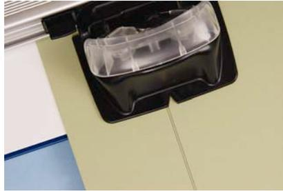
*V Groove cutting with the Trio System*
