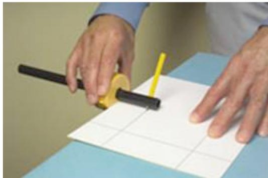
Overlap the mountboard blank facedown just over the edge of the work-surface. Having set the measurement of the Marker Gauge to the required width for the border and draw four lines on the back - the mountboard blank is now ready for cutting the bevel window
