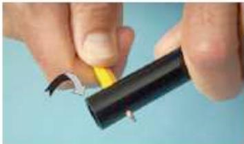
Insert the pencil into the hole in the shaft with a firm rotating and pushing action
