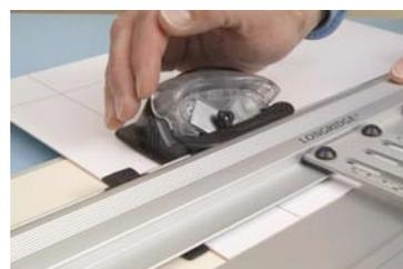
Manually retract the blade fully and take the cutter off the Trio Guide Rail. The cutter stops of course remain set for the opposite long side (if cutting a rectangle and for the other three sides if cutting a square mount). Turn the mount around and repeat the cut. Reset the bottom stop and repeat for the shorter sides if cutting a rectangular mount.
