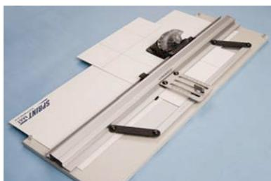
For larger mounts remove the Mount Stop and slide the mount blank up to the squaring pins instead
