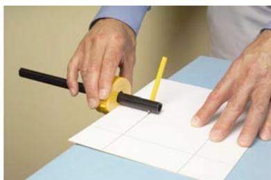
*place the mountboard on the worksurface just over the edge and keep the yellow block firmly up against the side of the mountboard when drawing the line*
