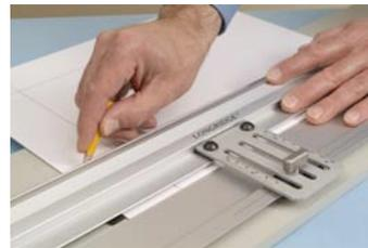
Place the Bevel Cutter onto the Trio Guide Rail and insert the two Cutter Stops. Before cutting, line up the centre of the V with the finish line and lock the top stop; slide the cutter back and line up the centre of the V with the start line and lock the bottom stop.
