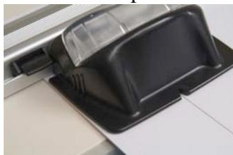
*the cutter stop is set by positioning the centre of the V on the intersecting line and then locking it in position*
