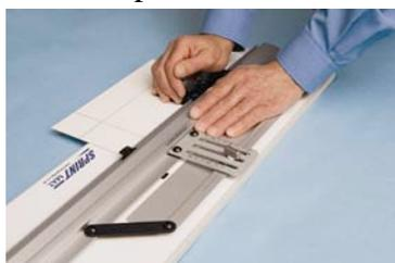
*ensure the SprintMat always supports both the rail and cutter*
