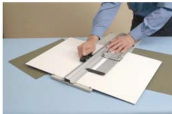
*be positive – don't hesitate, otherwise the blade may flex resulting in a curve at the end*
