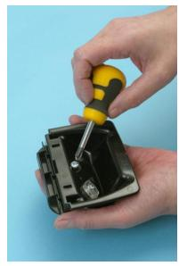
Turn anticlockwise to increase depth Turn clockwise to reduce depth
