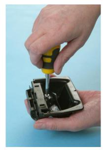
The blade depth of the cutter comes set for standard board (1.3mm / 1.4 mm). The thickness of mountboard does vary so you may need to fine tune the blade depth to suit the mountboard you are using.
