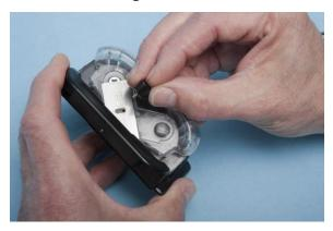
Step 2 – line up the hole in the blade with the screw hole underneath
