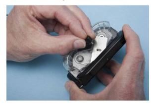
Step 2 – line up the hole in the blade with the screw hole underneath
