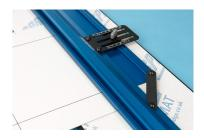
7. Place the bevel cutter onto the Guide Rail and insert the two Cutter Stops.
